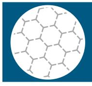
This unique lamination pattern ensures a strong bond between paper and foil, while forming air pockets to keep food insulated.
