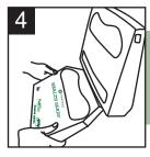
To avoid wasting any covers, envelope with remaining covers should be hung from hooks at bottom of dispenser (Secondary position), to have all covers used
