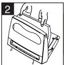
Place refill envelope in dispenser from top, lining it up with notches at bottom
